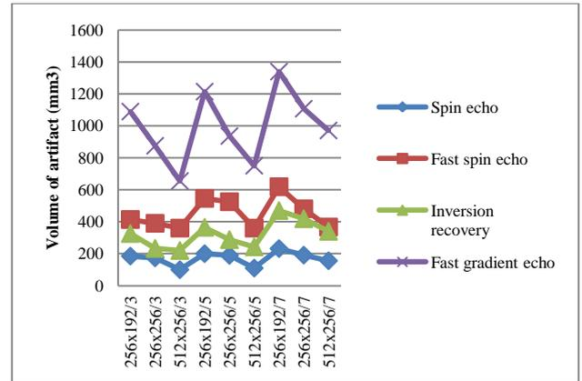
**Fig.1** The signal loss volume ( $\text{mm}^3$ ) versus pulse sequence, matrix size and slice thickness of volume of coil pack  $160 \text{ mm}^3$ .
