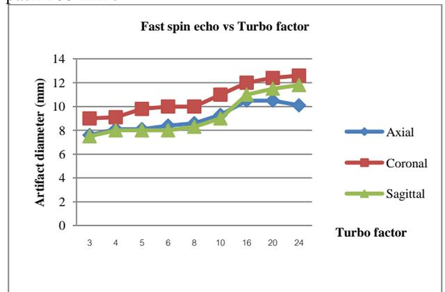
**Fig.2** The artifact diameter of fast spin echo versus turbo factor in three orthogonal planes. Coil packs maximum dimension 5.6x5.6x9.0 mm.
